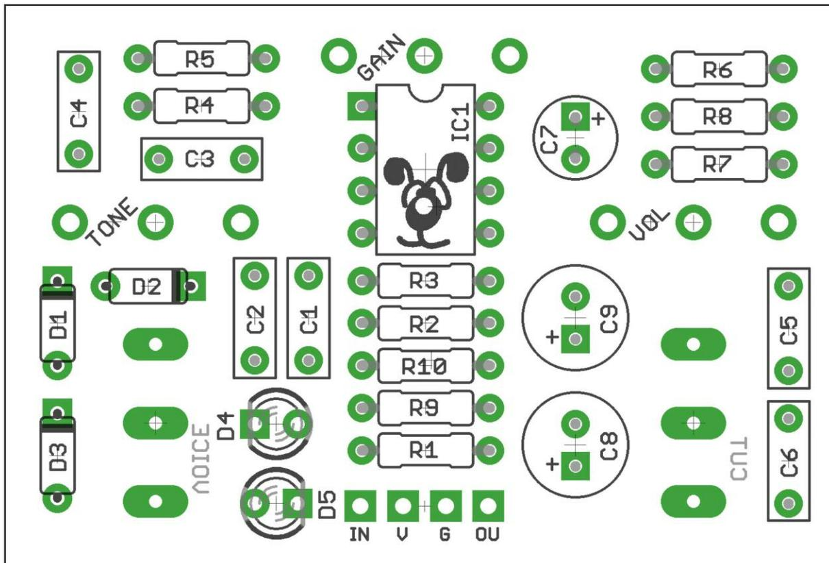
PCB layout ©2018 Pedal Parts Ltd.
