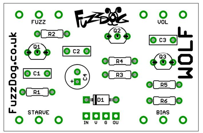
The power and signal pads on the PCB conform to the FuzzDog Direct Connection format, so can be paired with the appropriate daughterboard for quick and easy offboard wiring. Check the separate daughterboard document for details.
