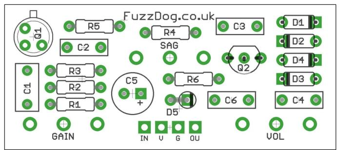
The power and signal pads on the PCB conform to the FuzzDog Direct Connection format, so can be paired with the appropriate daughterboard for quick and easy offboard wiring. Check the separate daughterboard document for details.
