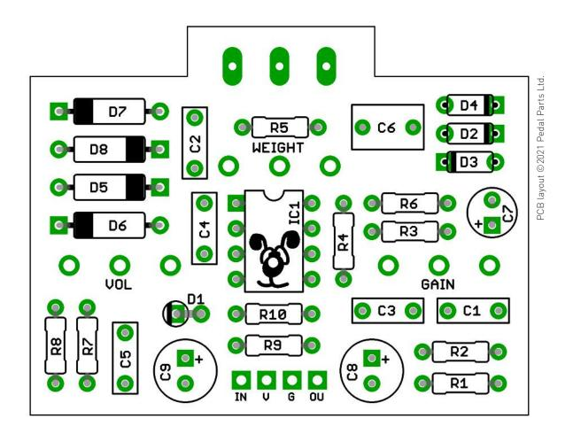
The power and signal pads on the PCB conform to the FuzzDog Direct Connection format, so can be paired with the appropriate daughterboard for quick and easy offboard wiring. Check the separate daughterboard document for details.
