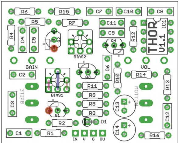
There are extra pads provided for the trimmers so you can use several different types. Just drop the pins into the holes as they naturally fall. Lines shown above show which pads are internally connected on the PCB.
