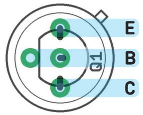
The outline for the smaller transistor shown is the correct orientation for 2N3904, 2N5088 etc.
