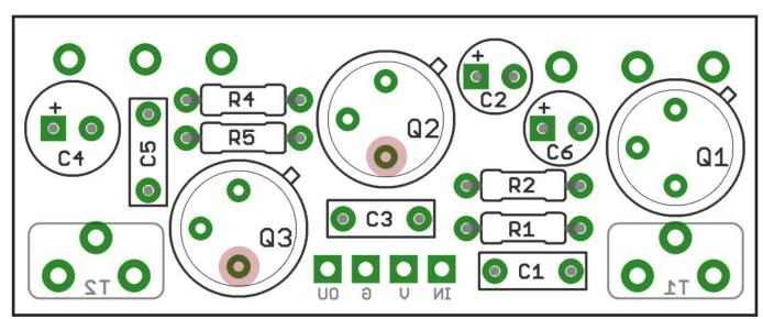
The power and signal pads on the PCB conform to the FuzzDog Direct Connection format, so can be paired with the appropriate daughterboard for quick and easy offboard wiring. Check the separate daughterboard document for details.
