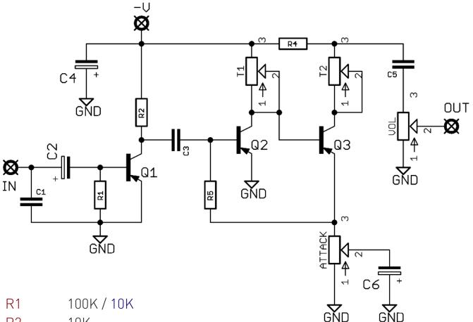
R2 10K R4 470R R5 100K C1 10n / 15n C2 4.7u / 10u С3 100n C4 47u C5 10n / 15n 4.7u / 10u C6 Q1,2,3 **PNP** Germaniums ATTACK 1KB VOL 100KA 100K preset T1 T2 10K preset
