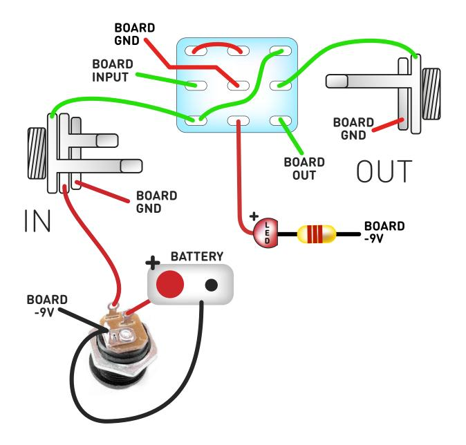
Wiring shown above will disconnect the battery when you remove the jack plug from the input, and also when a DC plug is inserted.
