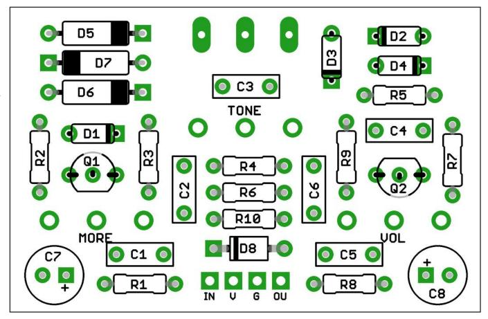
The power and signal pads on the PCB conform to the FuzzDog Direct Connection format, so can be paired with the appropriate daughterboard for quick and easy offboard wiring. Check the separate daughterboard document for details.
