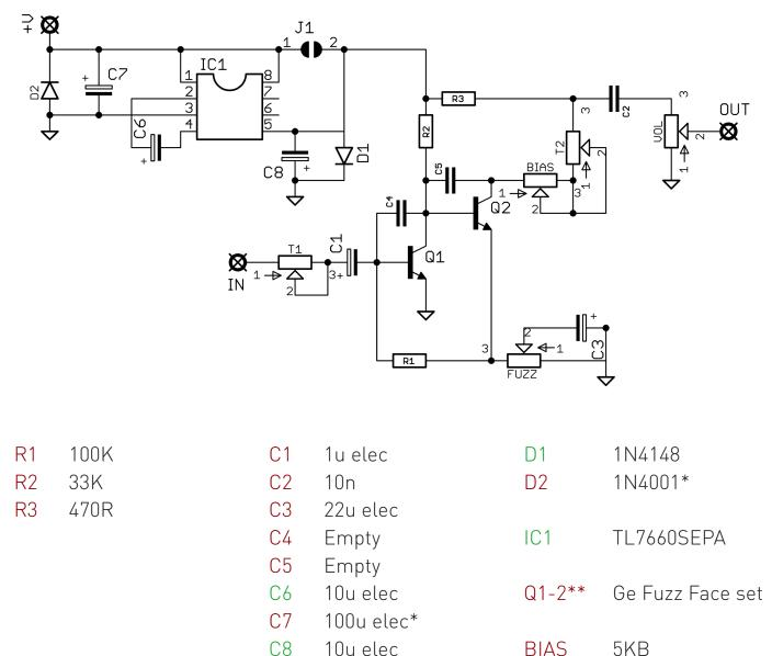
Parts listed in green are the optional voltage inverter. If you're not adding this leave these out and connect the pads on the back of the board as detailed on the previous page with a blob of solder.
