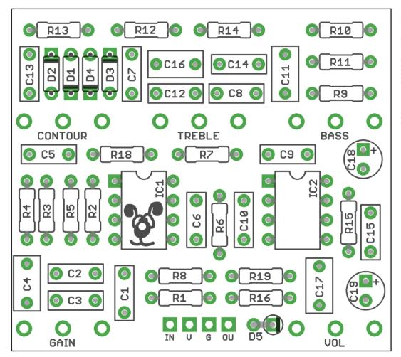
The power and signal pads on the PCB conform to the FuzzDog Direct Connection format, so can be paired with the appropriate daughterboard for quick and easy offboard wiring.
