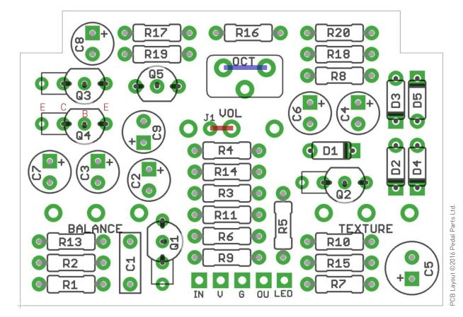
Place a jumper wire across the OCT trimmer pads as shown in blue above.
