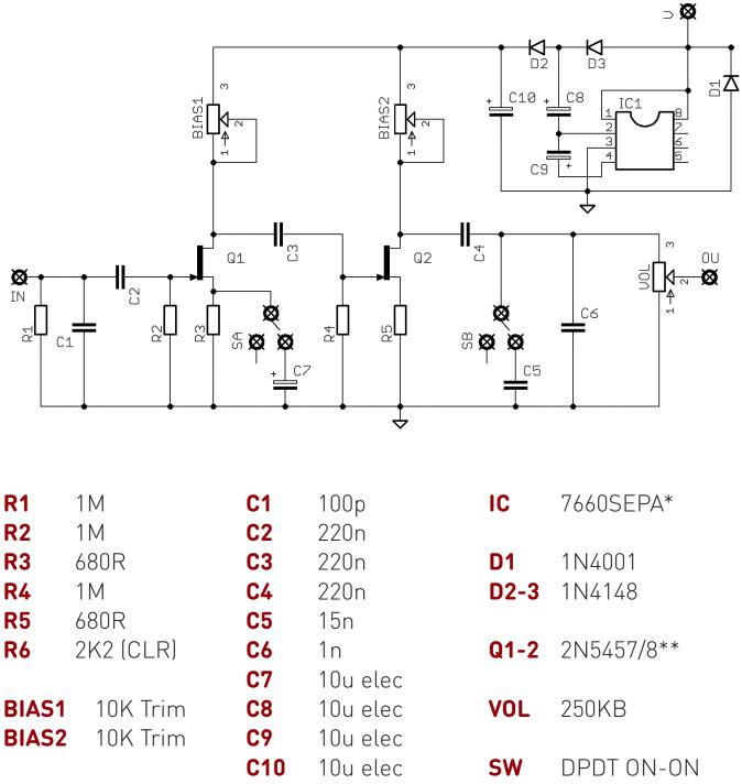
\*It's important to get a 7660 charge pump with an 'S' suffix to ensure it operates outside the audible frequency range, otherwise you will hear a whining noise from the output. A MAX1044 will also work. We exclusively use 7660SEPA from Microchip.
