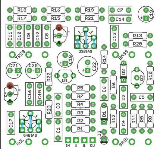
There are extra pads on trimmers to allow different package formats to be used. Pads are connected via PCB traces as shown above, so just fit your trimmer into whichever holes it fits naturally into. As long as you have one pin each in the left, centre and right sections. No jumpers are required.
