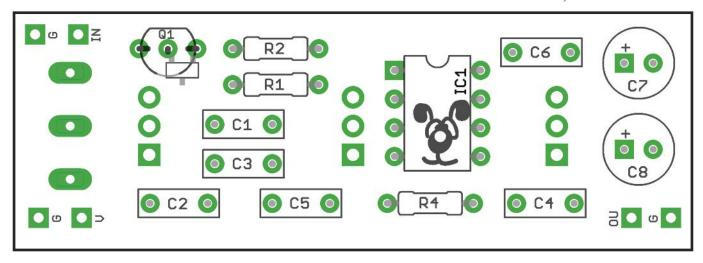
Be very careful when soldering Q1. FETs are very sensitive to heat. You should use some kind of heat sink (crocodile clip or reverse action tweezers) on each leg as you solder them. Keep exposure to heat to a minimum (under 2 seconds). Same goes for the IC if you aren't using a socket.
