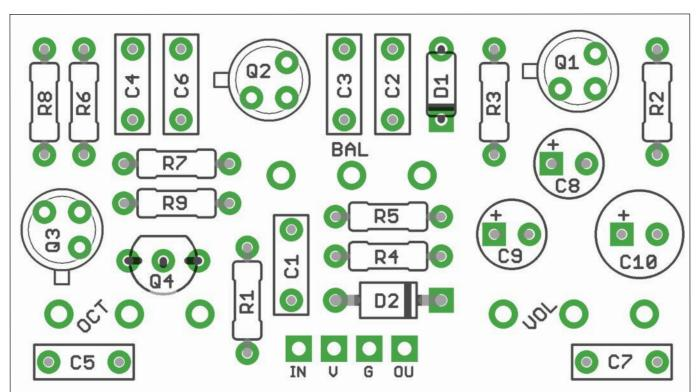
The power and signal pads on the PCB conform to the FuzzDog Direct Connection format, so can be paired with the appropriate daughterboard for quick and easy offboard wiring. Check the separate daughterboard document for details.
