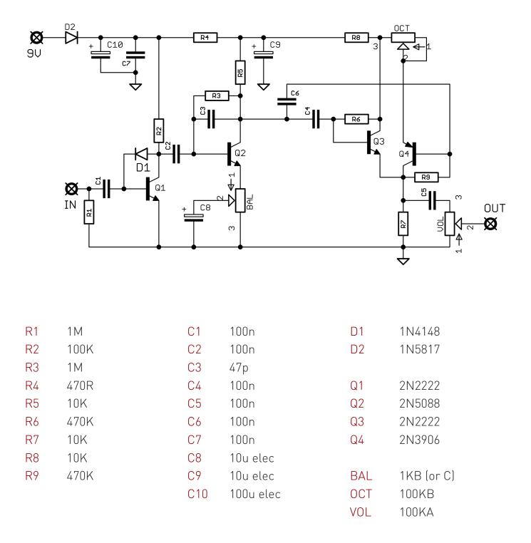
Feel free to play around with the transistors. Q1-3 are NPN, Q4 is PNP. 2N3904 will work well in Q3. We used the wrong footprint for Q2, so place it as shown in the cover image.
