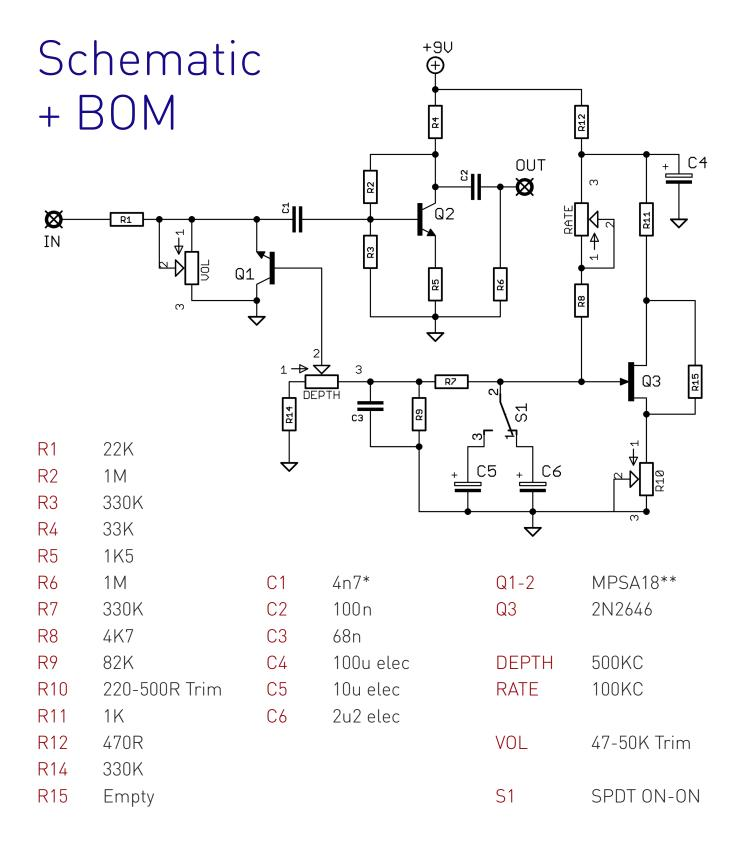
This BOM represents a build using the 2N2646 UJT. These are getting scarce. See page 5 for an alternative build using the readily available 2N6027 PUT.
