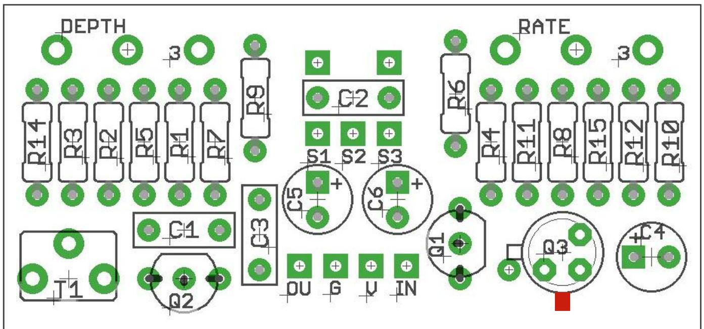
PCB Layout ©2015 Pedal Parts Ltd.
