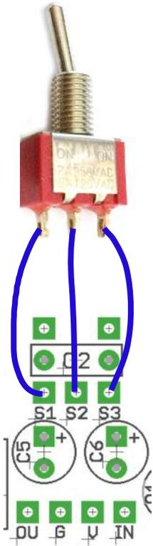
If you're using a wired switch, connect as shown. Ignore the two pads above C2 - they're only there as extra support for the board-mounted micro-toggle.
