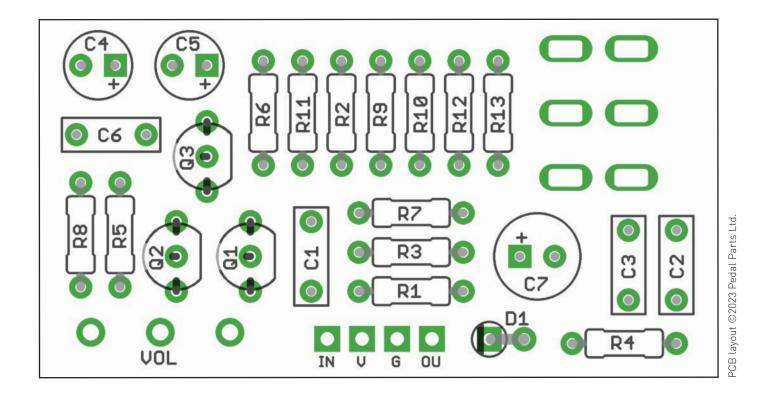
The power and signal pads on the PCB conform to the FuzzDog Direct Connection format, so can be paired with the appropriate daughterboard for quick and easy offboard wiring. Check the separate daughterboard document for details.
