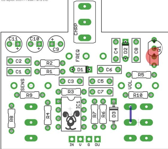
The power and signal pads on the PCB conform to the FuzzDog Direct Connection format, so can be paired with the appropriate daughterboard for quick and easy offboard wiring. Check the separate daughterboard document for details.
