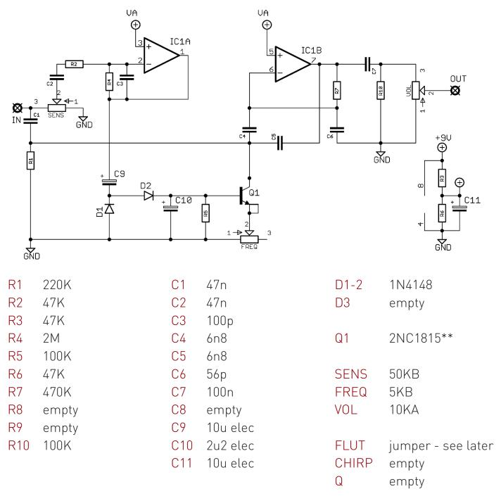
\*\*Other BJTs will work, and we've included pads to take standard CBE pinouts. See later in the doc for positioning for the 1815 which has a different pinout.
