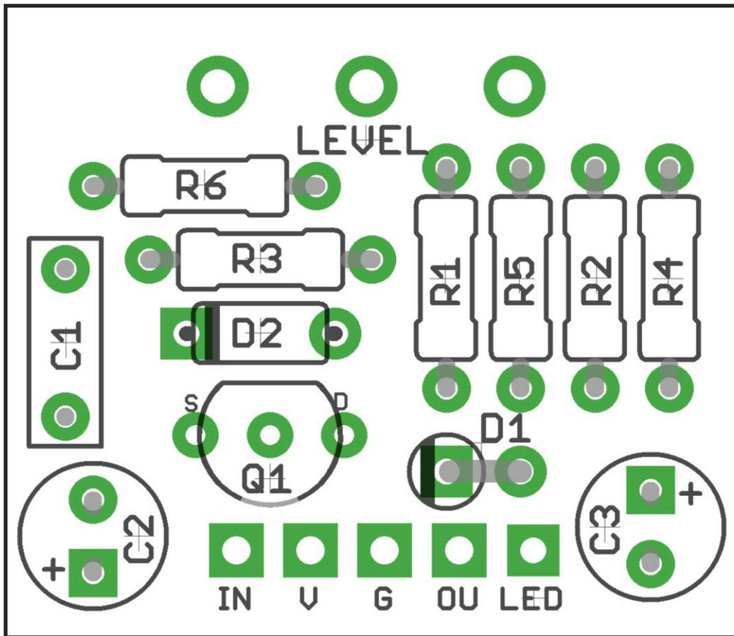
The power and signal pads on the PCB conform to the FuzzDog Direct Connection format, so can be paired with the appropriate daughterboard for quick and easy offboard wiring. Check the separate daughterboard document for details.
