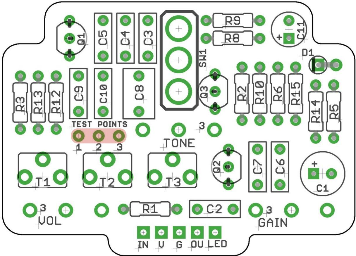
The power and signal pads on the PCB conform to the FuzzDog Direct Connection format, so can be paired with the appropriate daughterboard for quick and easy offboard wiring.
