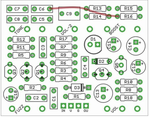
If using a ribbon cable you should solder it onto the component side of the PCB so it isn't interfering with the balance pot. Same goes for individual wires.
