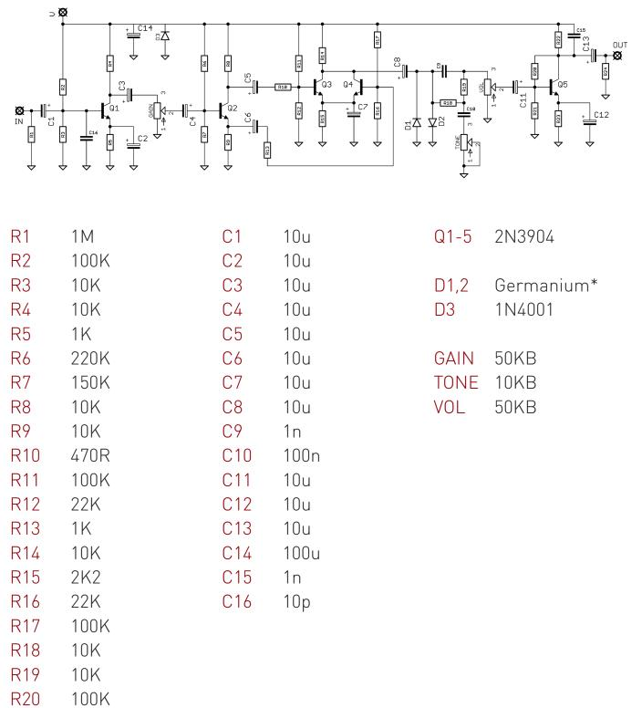
\*We supply Russian D9E diodes for D1-2. These have the stripes indicating the anode rather than cathode, so should be reversed compared to the silkscreen on the PCB. Refer to the image on the first page.
