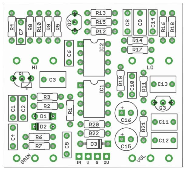
PCB layout ©2023 Pedal Parts Ltd.
