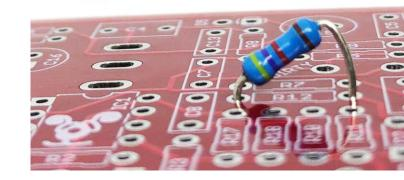
If you want to hide the hack you can just attach a wire between pads on the underside of the PCB. >>>
