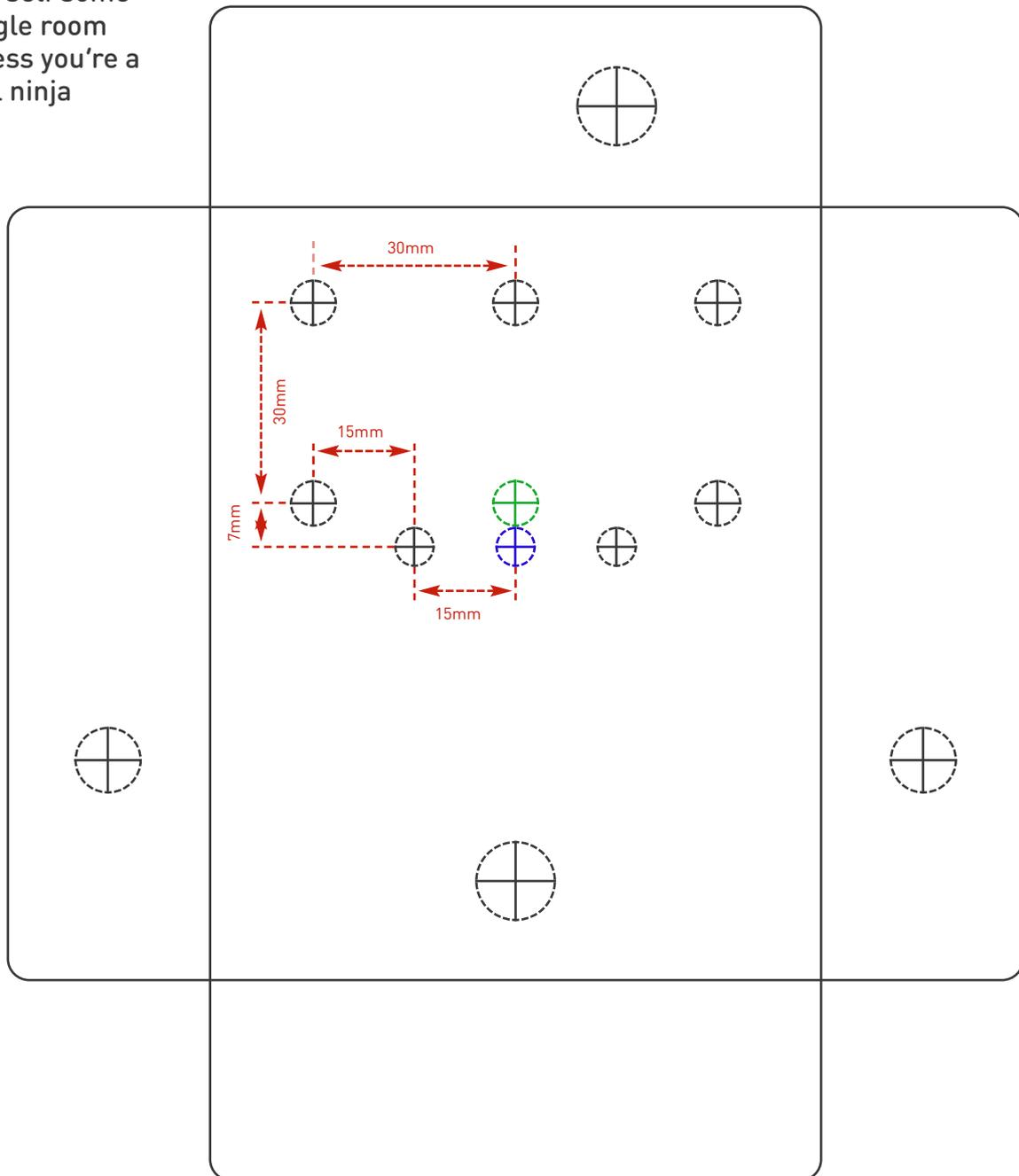
This template is a rough guide only. You should ensure correct marking of your enclosure before drilling. You use this template at your own risk. Pedal Parts Ltd can accept no responsibility for incorrect drilling of enclosures.
