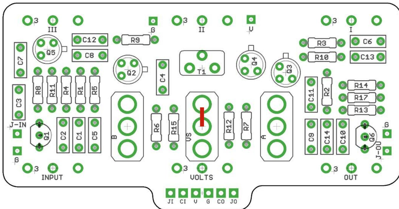
The power and signal pads on the PCB conform to the FuzzDog Direct Connection format, so can be paired with the appropriate daughterboard for quick and easy offboard wiring. If you use a 6-way connection cable you can choose to take your jack connections from the main PCB or the daughterboard. It's up to you. If you're not using a daughterboard ignore the J-IN and J-OUT connectors - they won't attach to anything without the daughterboard.
