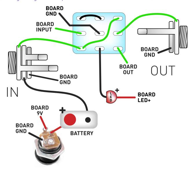
This circuit is standard, Negative GND. Your power supply should be Tip Negative / Sleeve Positive. That's the same as your standard pedals (Boss etc), and you can safely daisy-chain your supply to this pedal.
