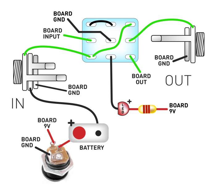
Wiring shown above will disconnect the battery when you remove the jack plug from the input, and also when a DC plug is inserted.
