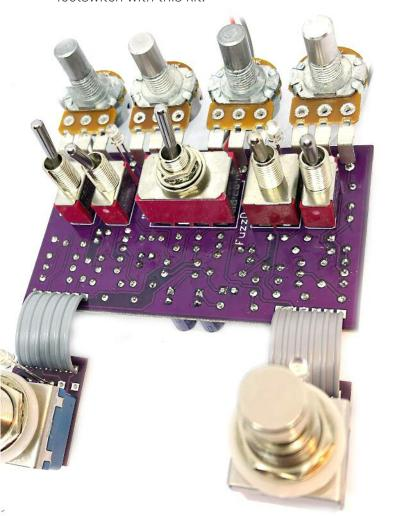
Be very careful when soldering the diode, transistors and LEDs. They're very sensitive to heat. You should use some kind of heat sink (crocodile clip or reverse action tweezers) on each leg as you solder them. Keep exposure to heat to a minimum (under 2 seconds). The same goes for the IC if you aren't using a socket.
