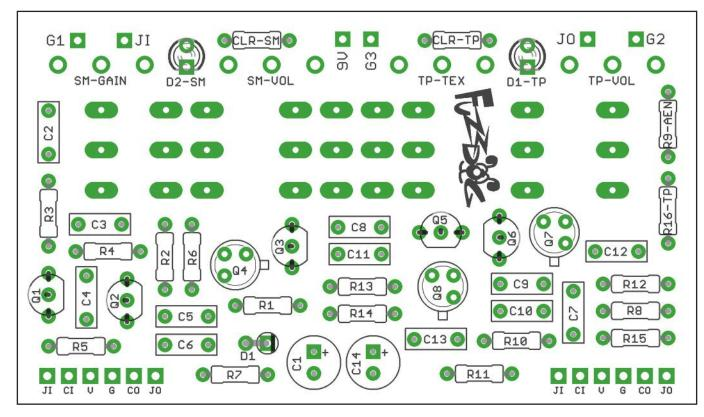
The power and signal pads on the PCB conform to the FuzzDog Direct Connection format, so can be paired with the appropriate daughterboard for quick and easy offboard wiring. Check the separate daughterboard document for details. We supply daughterboards with LED above the footswitch with this kit.
