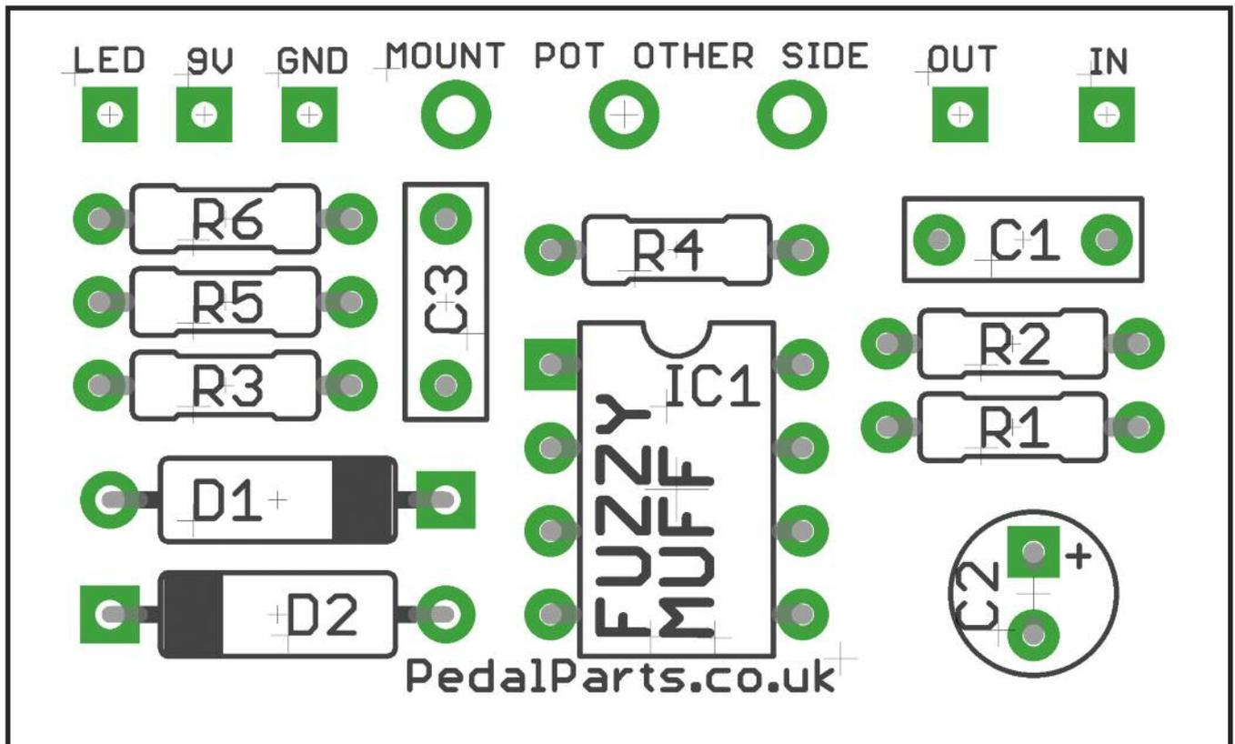
The PCB is designed to have the volume pot mounted directly to it. You can use wire if you like - simply connect the board pads to the corresponding pins on the pot.
