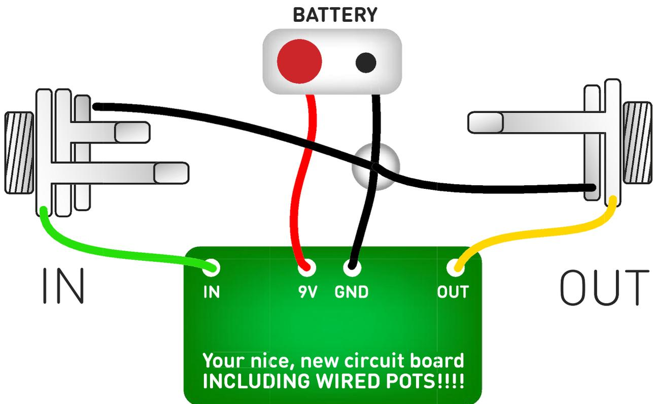
Once you've finished the circuit it makes sense to test it before starting on the switch and LED wiring. It'll cut down troubleshooting time in the long run. If the circuit works at this stage, but it doesn't once you wire up the switch - guess what? You've probably made a mistake with the switch.
