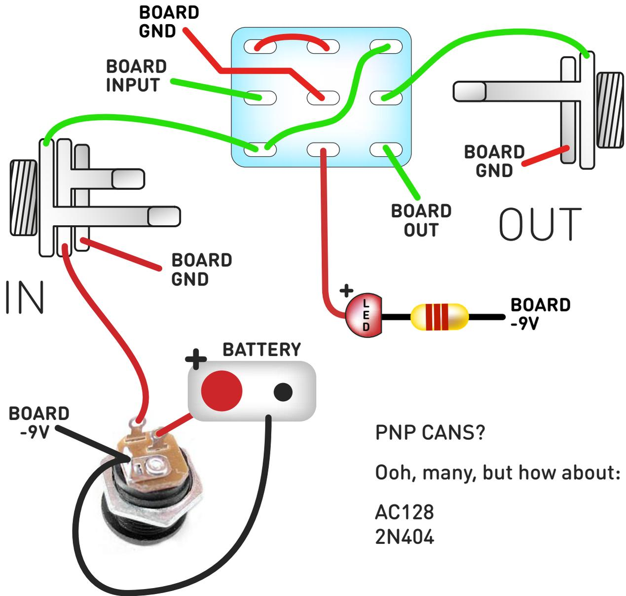
The Board GND connections don't all have to directly attach to the board. You can run a couple of wires from the DC connector, one to the board, another to the IN jack, then daisy chain that over to the OUT jack.
