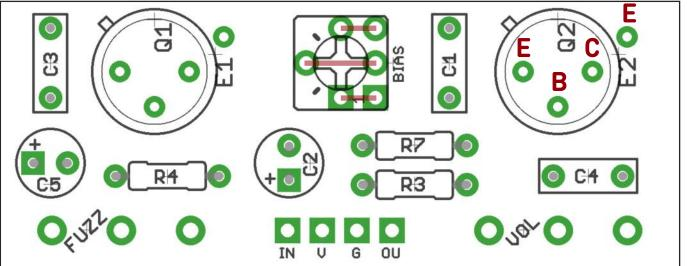
The power and signal pads on the PCB conform to the FuzzDog Direct Connection format, so can be paired with the appropriate daughterboard for quick and easy offboard wiring. Check the separate daughterboard document for details.
