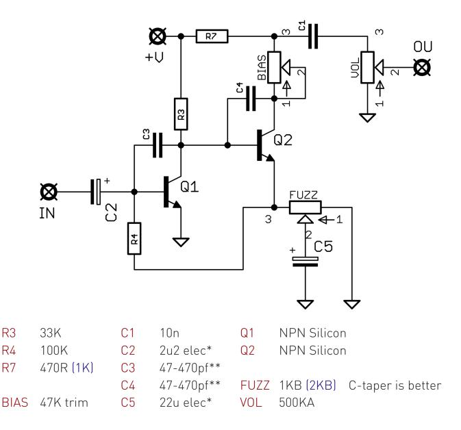
Silicon version, along with a couple of value swaps (brackets) for the Mayer modified version which is a bit louder and has a better range on the Fuzz control.
