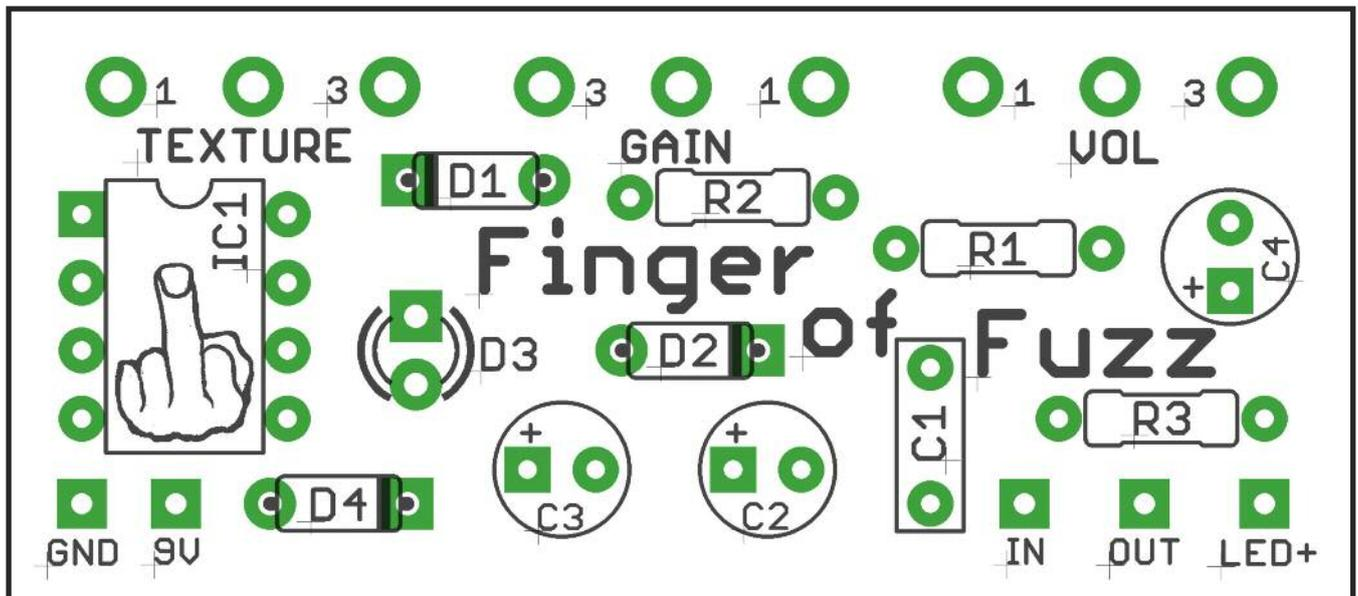
The PCB is designed to have the pots mounted directly to it. You can use wire if you like - simply connect the board pads to the corresponding pins on the pots.
