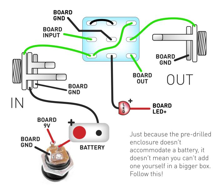
There are GND connections for both jacks at either end of the board.
