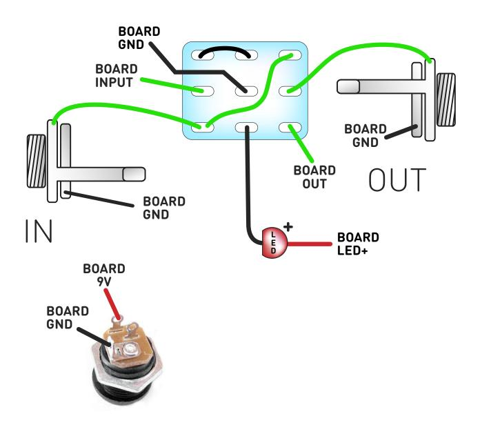
There are GND connections for both jacks at either end of the board.
