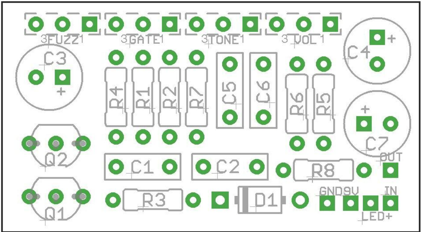
A teeny oops - the OUT label overlaps the pad on the board - there it is under C7.
