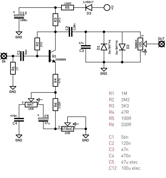
Feel free to experiment with substitutions, especially for Q1 and the clipping diodes D1-2.
