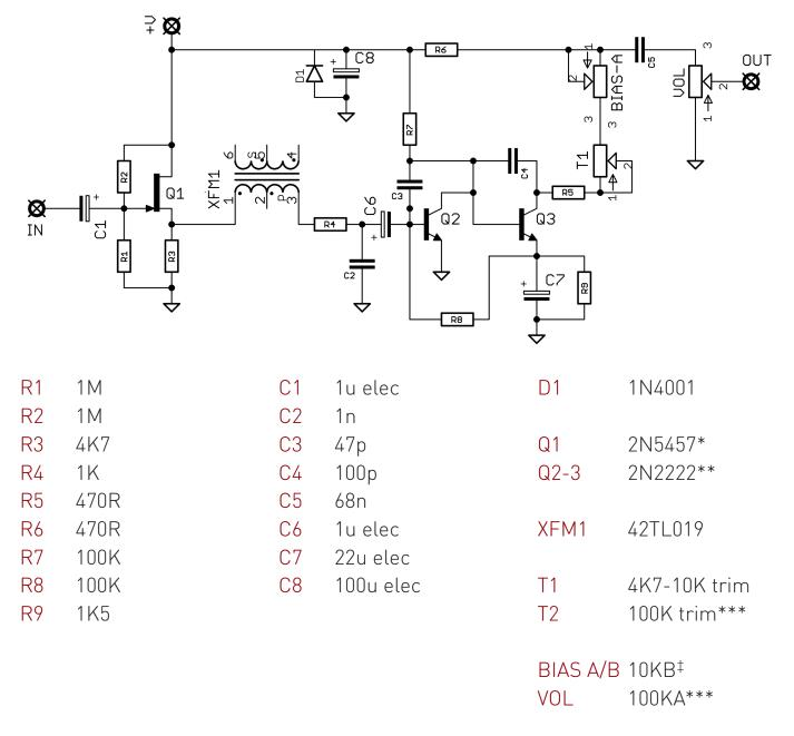
\*Original uses PF5102. It makes no difference at all to the sound. Pads are provided for through-hole or SMT FETs. The SMT version of 2N5457 is MMBF5457.
