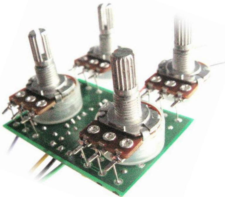
The pads for the pots are spaced so you can use vertical pots if you wish. Why not try "Cheating Verticals" by soldering snipped component legs to the pots as shown left. You can just wire them normally though.
