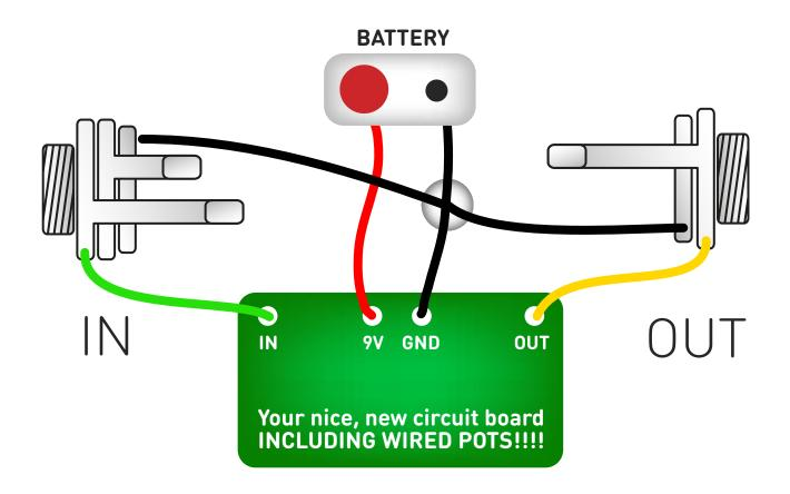
Once you've finished the circuit it makes sense to test is before starting on the switch and LED wiring. It'll cut down troubleshooting time in the long run. If the circuit works at this stage, but it doesn't once you wire up the switch - guess what? You've probably made a mistake with the switch.
