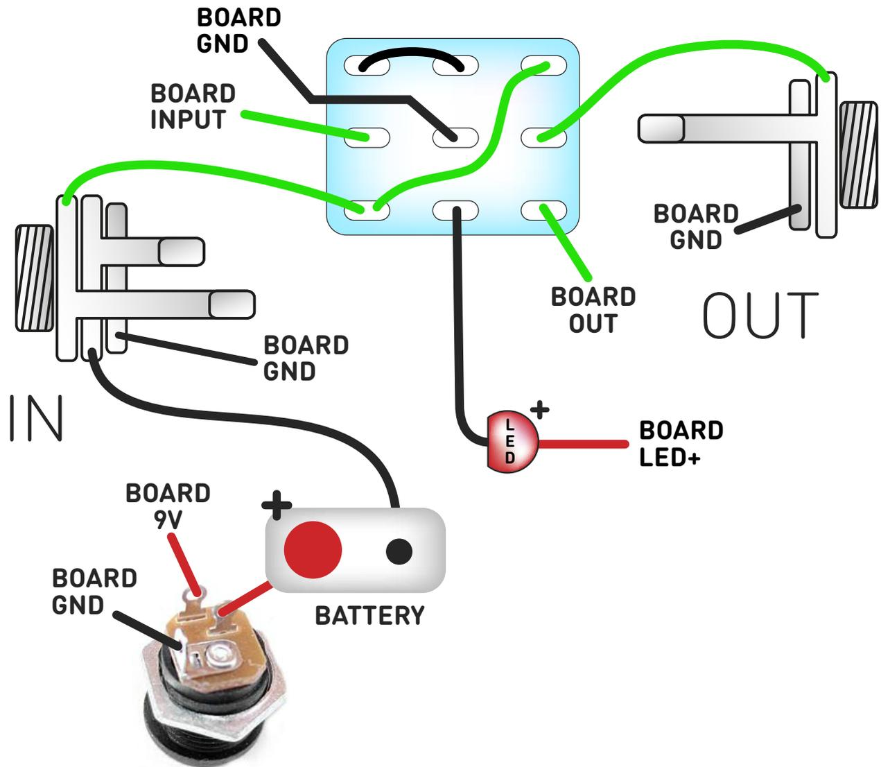
The Board GND connections don't all have to directly attach to the board. You can run a couple of wires from the DC connector, one to the board, another to the IN jack, then daisy chain that over to the OUT jack. It doesn't matter how they all connect, as long as they do.
