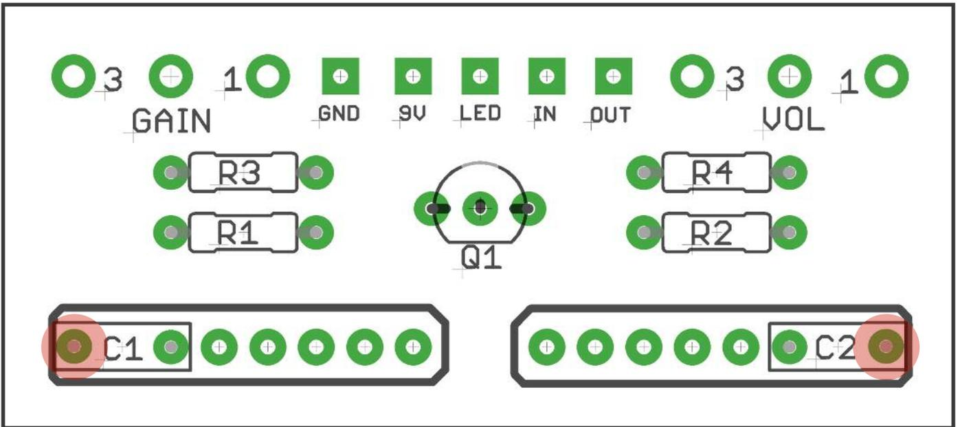
The PCB has extra pads for C1 and C2 to allow different sized caps to be used with ease. As long as one leg of each cap goes into the shaded holes shown above, the other leg can go into any of the other pads belonging to each cap.
