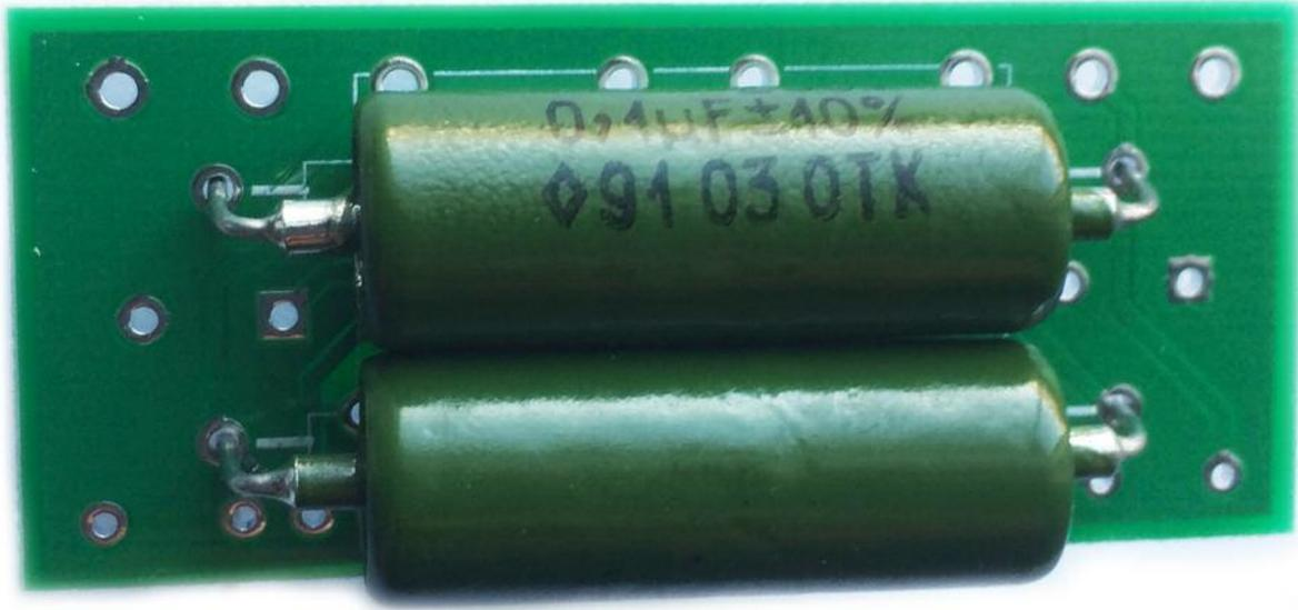
You'll notice there are extra pads next to C1 and C2. These allow easy use of bigger caps than standard 5mm pitch. If using them, make sure one leg of your cap goes into the pad nearest the side of the board, then the other leg can go in any of the other three pads at the other end of the cap space. If you look at the board layout on the previous page, the pads marked in blue all connect together at one end of C1, ditto the red ones and C2.
