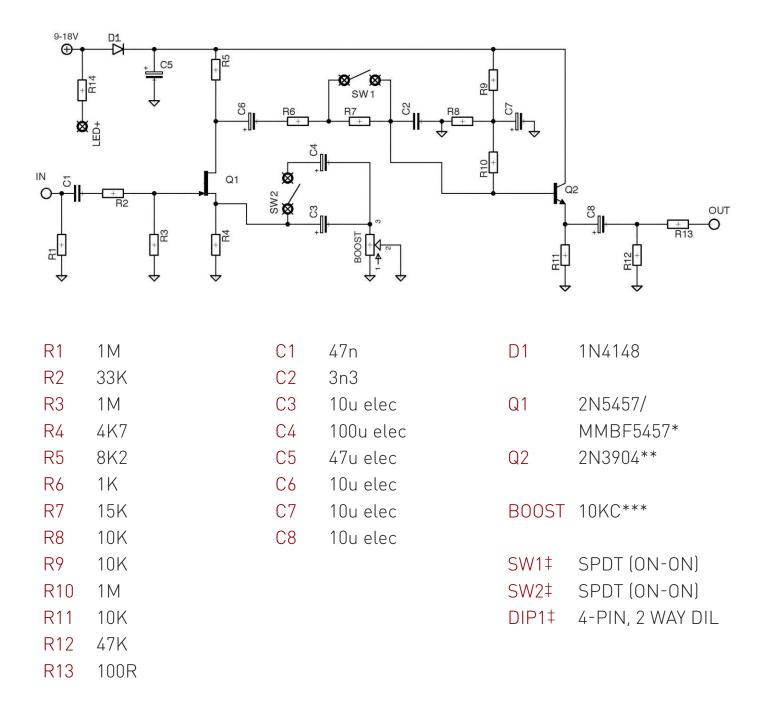
\*The PCB is designed for through-hole or SMT FET.
