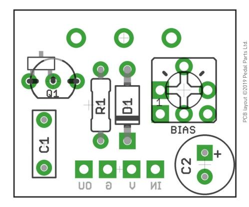
The board has been designed to take a through-hole or SMT FET.
