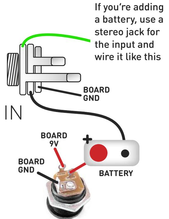
The Board GND connections don't all have to directly attach to the board. You can run a couple of wires from the DC connector, one to the board, another to the IN jack, then daisy chain that over to the OUT jack.
