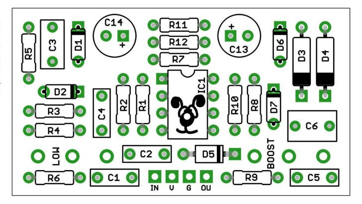
The power and signal pads on the PCB conform to the FuzzDog Direct Connection format, so can be paired with the appropriate daughterboard for quick and easy offboard wiring. Check the separate daughterboard document for details.
