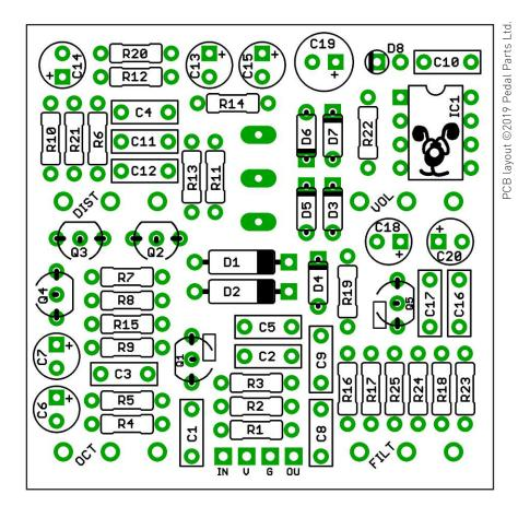
The power and signal pads on the PCB conform to the FuzzDog Direct Connection format, so can be paired with the appropriate daughterboard for quick and easy offboard wiring. Check the separate daughterboard document for details.
