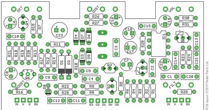
Two of the power and signal pads on the PCB conform to the FuzzDog Direct Connection format, so can be paired with the appropriate daughterboard for quick and easy offboard wiring. Check the separate daughterboard document for details. The optional Octave-Bypass pads need to be wired differently, but a daughterboard can still be used.
