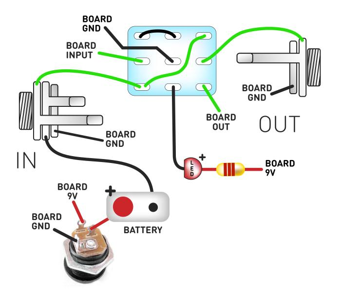
Wiring shown above will disconnect the battery when you remove the jack plug from the input, and also when a DC plug is inserted.
