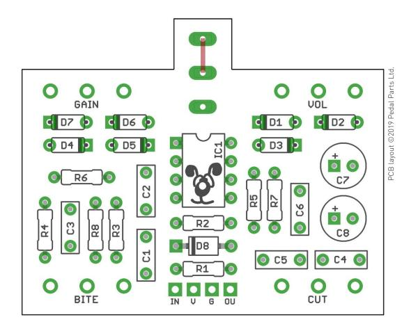
The power and signal pads on the PCB conform to the FuzzDog Direct Connection format, so can be paired with the appropriate daughterboard for quick and easy offboard wiring. Check the separate daughterboard document for details.
