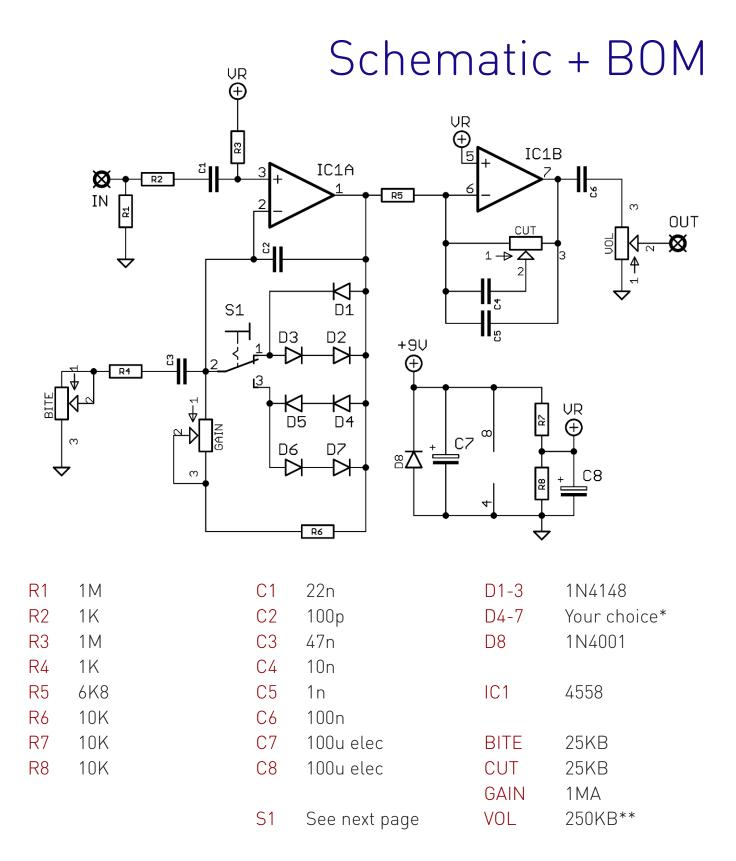
\*There are extra spots for a second set of clipping diodes. Try whatever you like in any configuration. If you are adding this option you'll need to put a SPDT toggle switch in S1.
