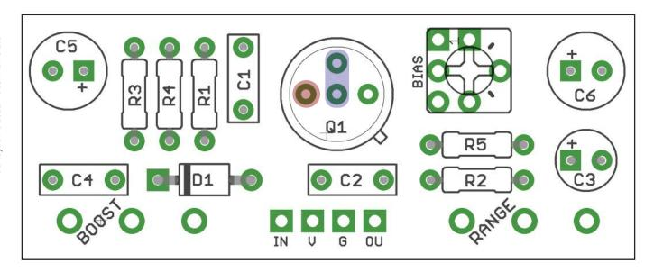
The power and signal pads on the PCB conform to the FuzzDog Direct Connection format, so can be paired with the appropriate daughterboard for quick and easy offboard wiring. Check the separate daughterboard document for details.
