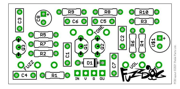
The power and signal pads on the PCB conform to the FuzzDog Direct Connection format, so can be paired with the appropriate daughterboard for quick and easy offboard wiring. Check the separate daughterboard document for details.
